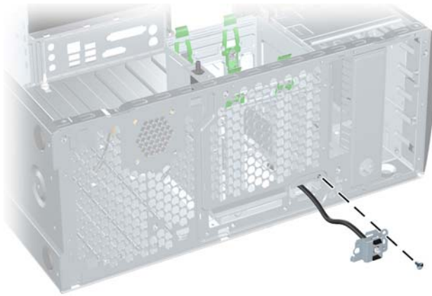
Figure 4-12 Removing the power button
