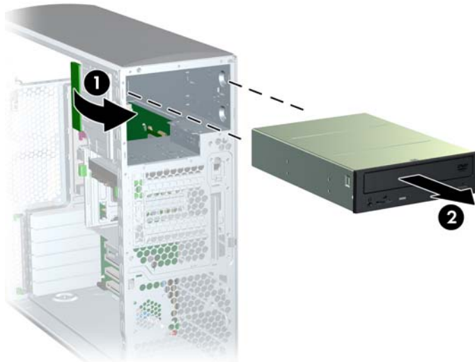
Figure 4-34 Removing the optical drive from the chassis
