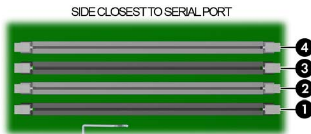
Figure 4-19 Identifying the memory slots
