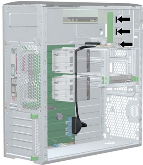
Figure 4-38 Routing the diskette drive cable to the system board
