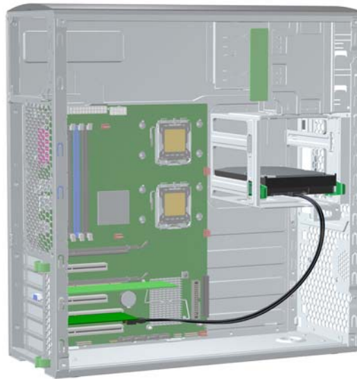
Figure 4-43 Connecting data cable to SAS controller card
